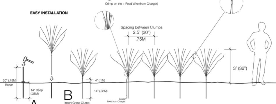
With a 30" piece of 3/8" Rebar Hammer a 14" deep pilot hole TOTALHABITAT.COM
